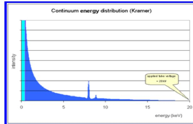
Besides the K- and L-lines of the Rh-anode this spectrum shows the continuous Bremsstrahlung too. This radiation is important for the effective excitation of all elements in the sample. The low energy part of this radiation will be absorbed in the tube window.
