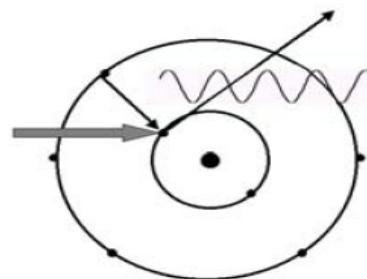
Electrons in the tube ionise a atom of the target-material.
